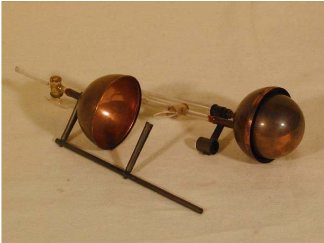
Figure 2. Original apparatus which Stefan used to evaluate the amount of heat lost in an experiment by Dulong and Petit.
